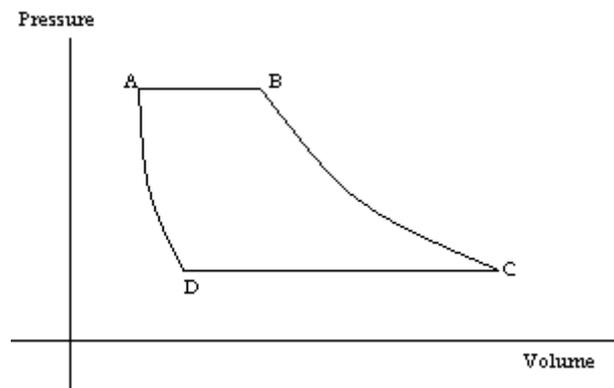
**Figure 2.9: Carnot's cycle for a steam engine**
