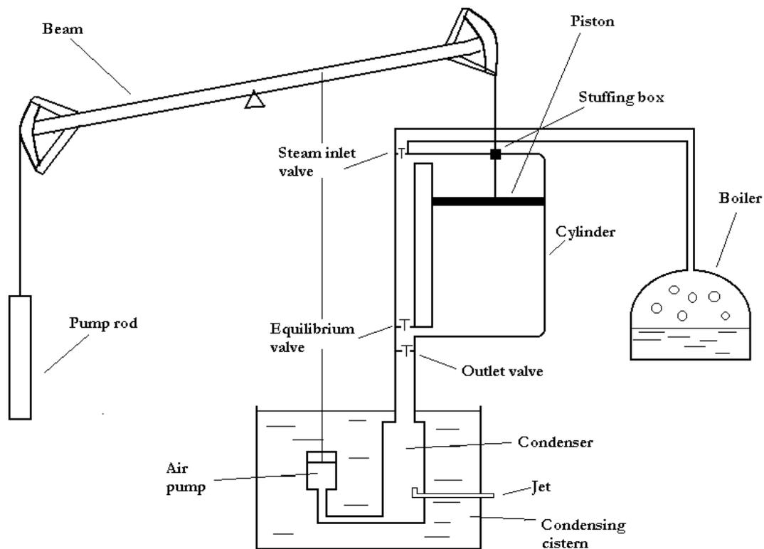
**Figure 2.5: The Watt pumping engine**
