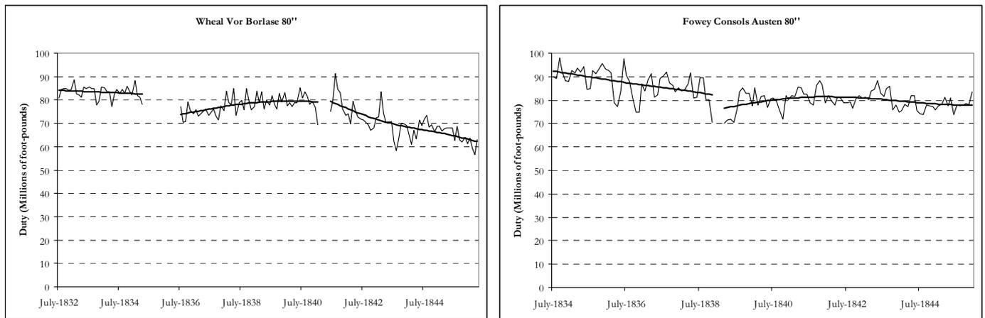
**Figure 7.14: Duty of Cornish engines (the 1830s)**
