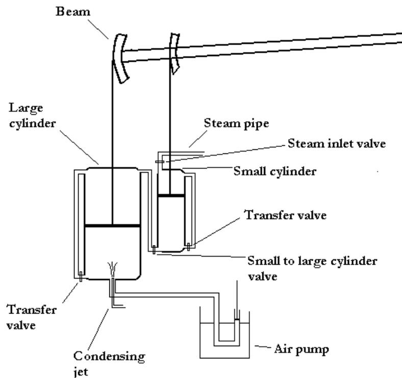
**Figure 2.8: The Hornblower compound engine**
