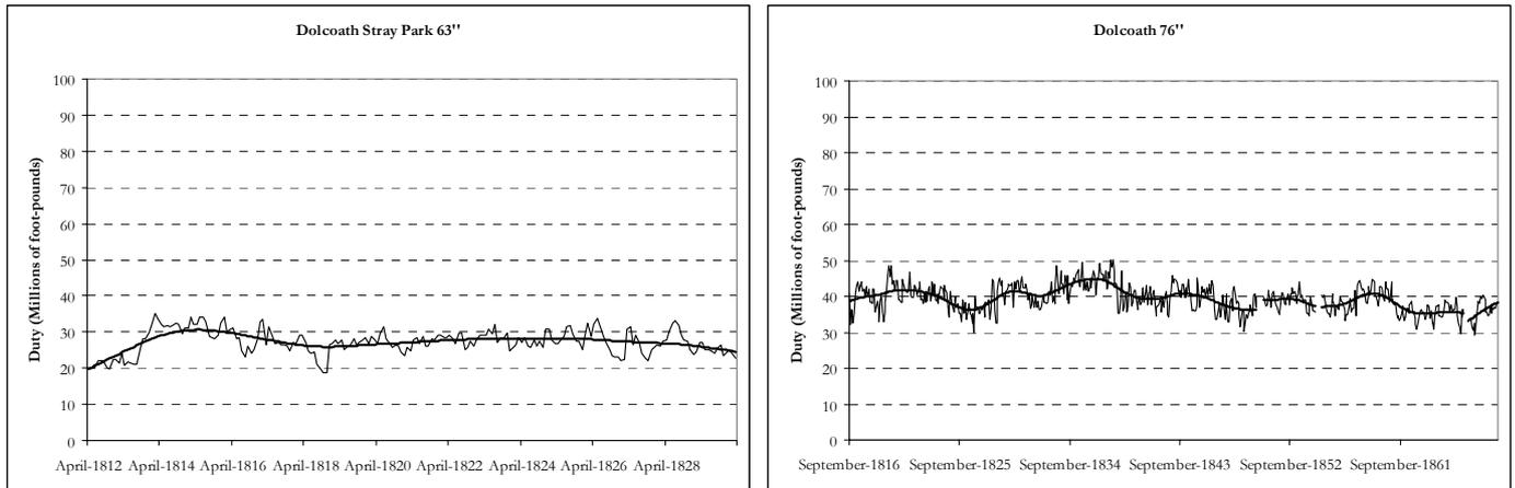
**Figure 7.9: Duty of Cornish engines (the emergence of the high pressure paradigm)**
