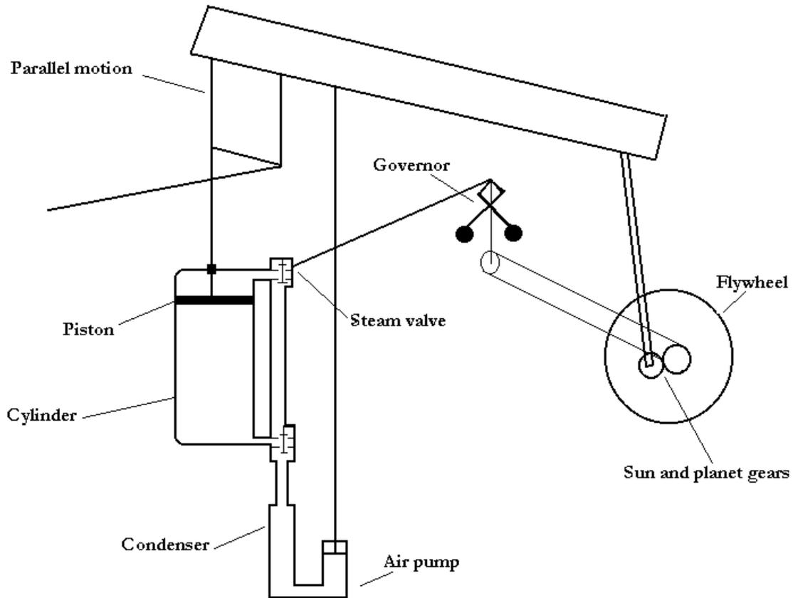
**Figure 2.6: The Watt double acting rotary engine**
