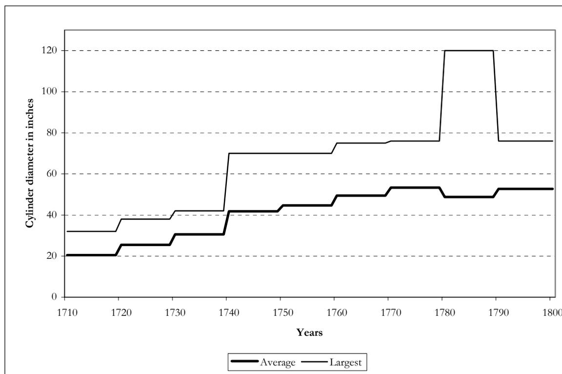
**Figure 2.4: Cylinder diameter of Newcomen engines, 1710-1800**
