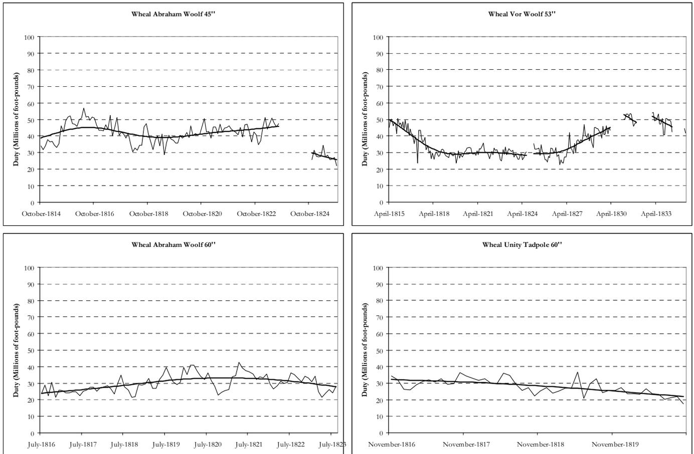
**Figure 7.10: Duty of Cornish engines (early compound engines designed by Arthur Woolf)**
