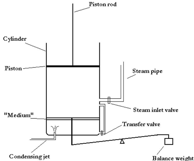
**Figure 2.7: The Symington pumping engine**
