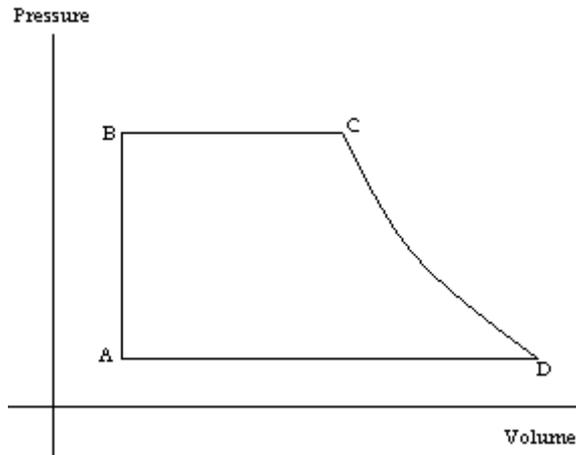
**Figure 2.10: Rankine's cycle for a steam engine**
