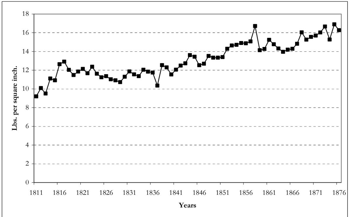
**Figure 6.20: Average load per square inch on cylinder, 1811-1876**
