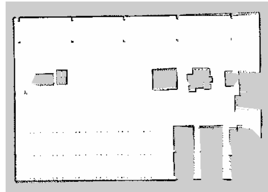
FIGURE 6. Occupancy Grid Map of the warehouse environment obtained using the GMapping algorithm.
