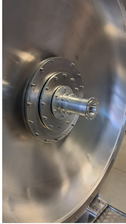
Figure 6: Setup with tube of aspect ratio 4 at the auxiliary chamber interface.
