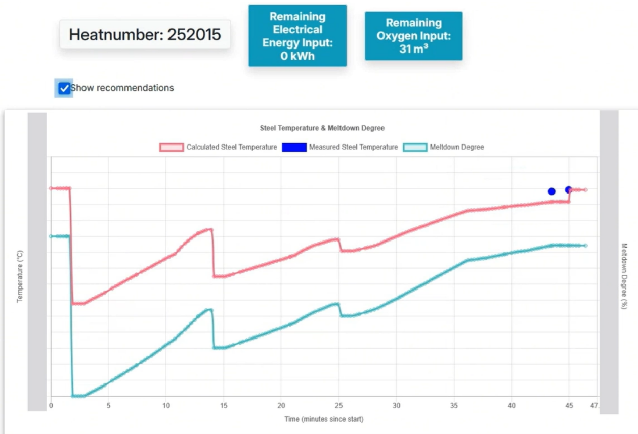
Figure 4. One of the views in EAF decision support, currently in endpoint control stage (some data hidden due to the corporate privacy and confidentiality policy)
