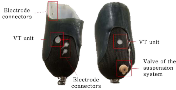
Fig. 8. Final soft socket with four sEMG sensors and three vibrotactile (VT) units (medial view, left; lateral view, right).
