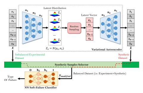
Fig. 2. Proposed approach: variational-autoencoder followed by a synthetic samples selector.
