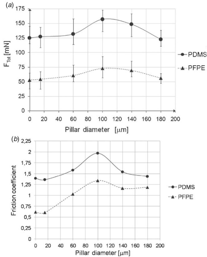
**Figure 9.** Friction force versus pillar diameter (a) and friction coefficient versus pillar diameter (b). The friction force was calculated for a load value of 0.6 N, which is the leg pulling force on the tissue.
