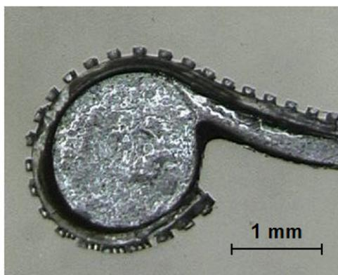
**Figure 3.** The leg covered with the polymeric pattern.
