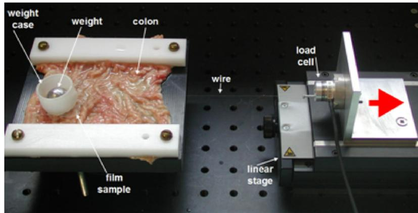
Figure 7. Friction experiments: set-up and typical curve.
