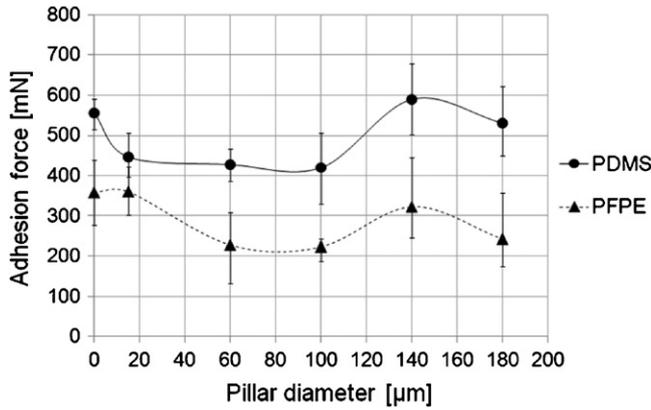
Figure 5. Graph of adhesion force versus pillar diameter.
