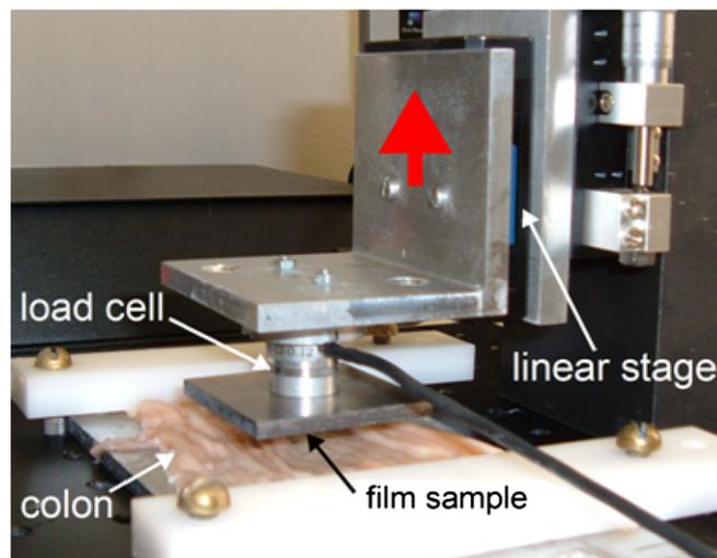
**Figure 4.** Adhesion experiments: set-up and typical curve.
