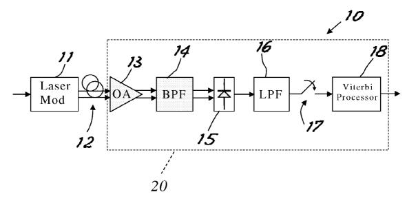
(57) Abstract: A method of and a receiver(20) for detection of a received signal in an optical fibre communication system using Viterbi algorithm methodology in which branch metrics are obtained using approximated expressions to calculate the branch metrics. Use of the expressions results in practically the same performance as a receiver based on exact metrics.
