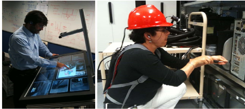
Figure 6 - The helper control console (left) and the worker wearable unit (right)
