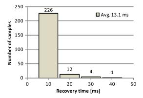
Fig. 6. Statistical distribution: recovery time [ms] measured in the experimental test bed.
