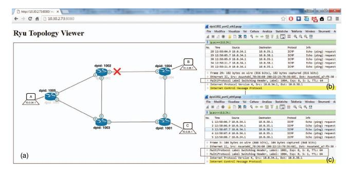
Fig. 5. SR-FAILOVER scheme test bed: (a) network topology visualized through the Ryu Topology Viewer web-based script; (b) Wireshark capture on port 2 of the node with dpid 1002; (c) Wireshark capture on port 3 of the node with dpid 1002.
