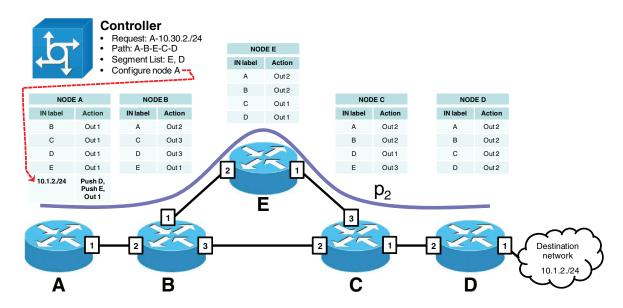
Fig. 1. SR operation example; all nodes are reported with the associated IP/MPLS forwarding table. In the figure, node A is configured by the controller to enforce  $\bar{p}_2$  with the actions push E, push D, out 1; actions to enforce  $\bar{p}_1$  are push D, out 1.
