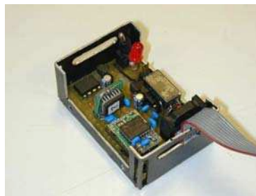
Fig. 1 The developed IMU, endowed with two dual-axis accelerometers and one single-axis gyro.
