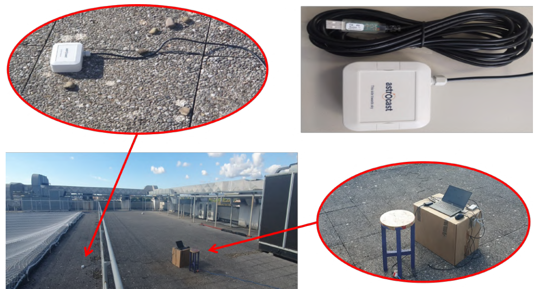
Figure 6. Setup of the live experiment (bottom left photo) using the Astronode S DevKit (upper right photo).
