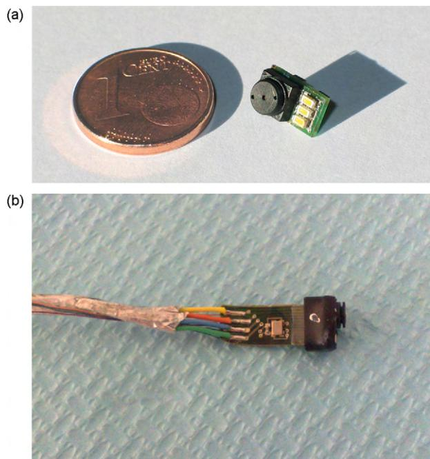
Fig. 1. The first prototype of the camera module, with its size compared to a €1 cent coin (a). A detail of camera cable (b).
