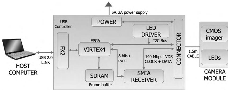
Fig. 2. Hardware architecture of the demonstration system.
