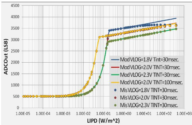
Fig. 9. Modeled and experimental power responsivity of the linear-logarithmic pixel at different  $V_{LOG}$  and  $T_{INT}$  values over the whole LIPD range.
