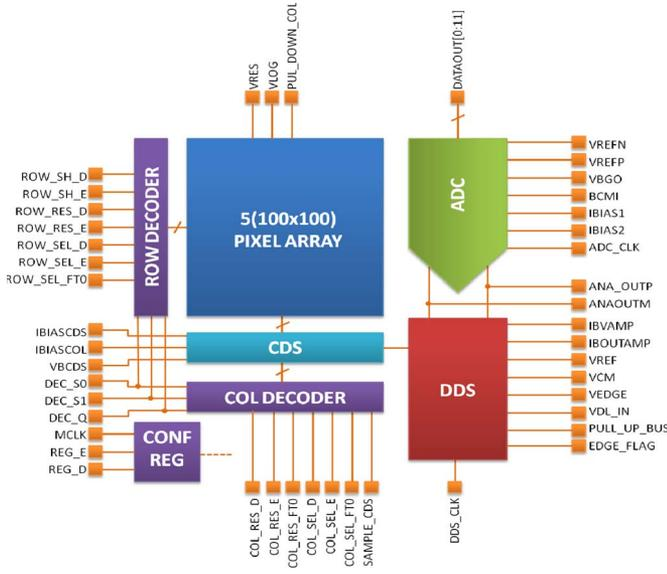
Fig. 3. Simplified block diagram of the camera.
