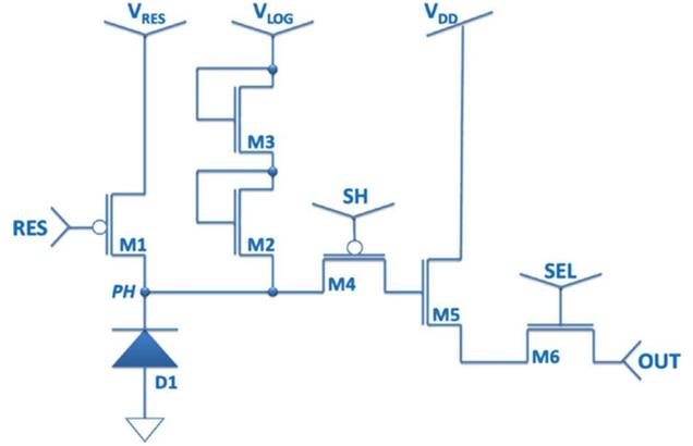
Fig. 1. Schematic of the linear-logarithmic pixel.
