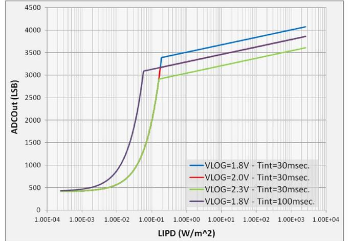
Fig. 2. Simulated power responsivity for the linear-logarithmic pixel at different  $V_{LOG}$  and  $T_{INT}$  values. ADCOUT is the ADC digital output word as defined in Section III.
