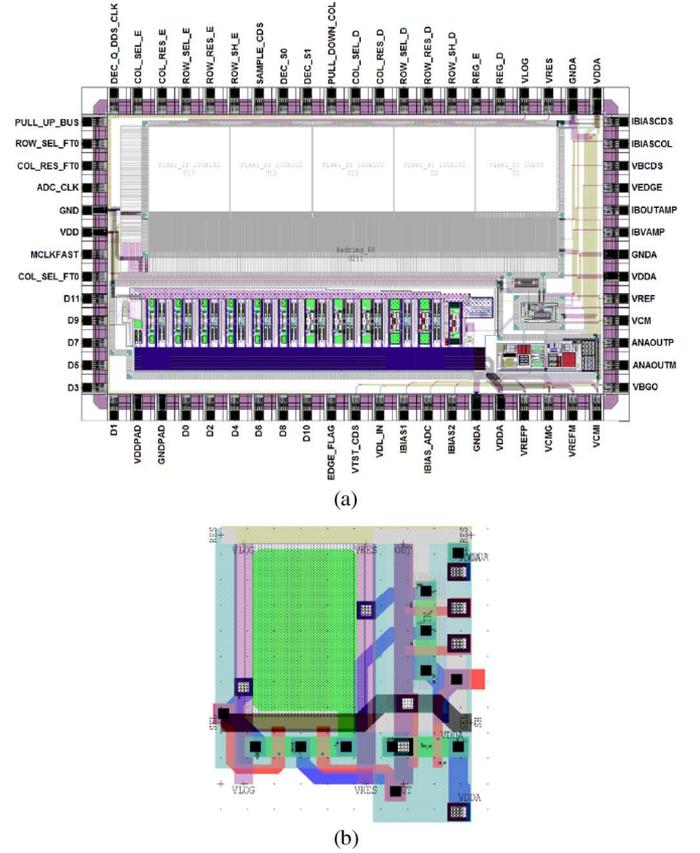
Fig. 4. Complete (a) imager and (b) pixel layout.
